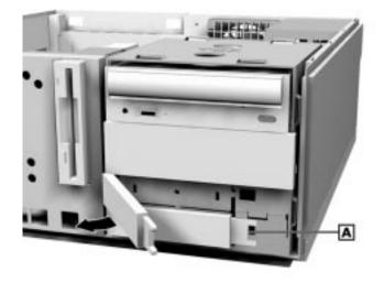
Removing the Blank Panel
